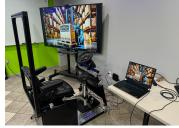
For those that want a more stationary system, Virtual Forklift Simulator provides an immersive simulator platform option for both the LIVE and the NEXUS systems. The classroom standard platform includes a standard forklift seat and a solid foundation for the controls and student comfort. In addition to the solid construction, the classroom standard includes the industries
